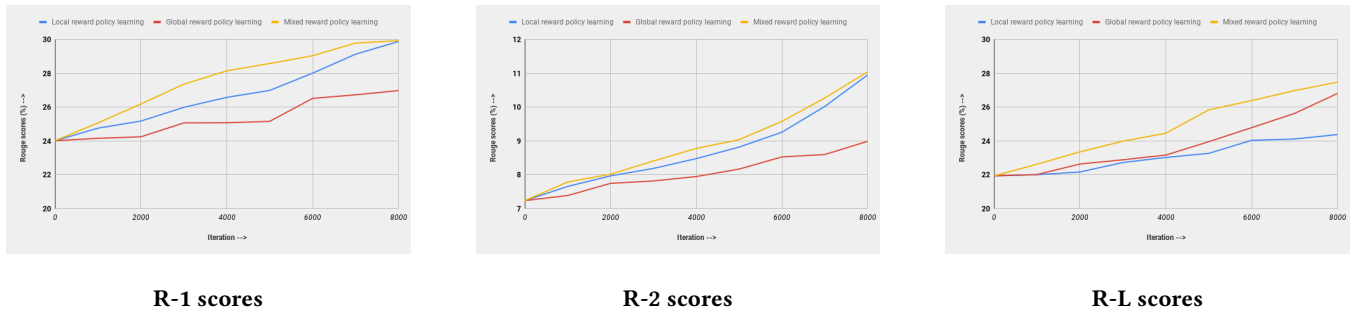
Figure 4: ROUGE score evaluation of the proposed methods during the training process. The Local rewards based method (Blue) has better R-1 and R-2 scores compared to Global rewards based method (Red). However, Global rewards based method (Red) has better in R-L score compared to Local rewards based method (Blue). Mixed reward based method (Yellow) has the best rouge scores in all categories.
